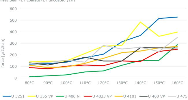
Heat Seal PET coated/PET uncoated (1K)
