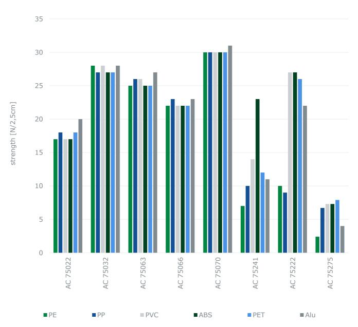
FINAT Test Method FTM 1, Coating Weight: 65 g/m<sup>2</sup>, dry
