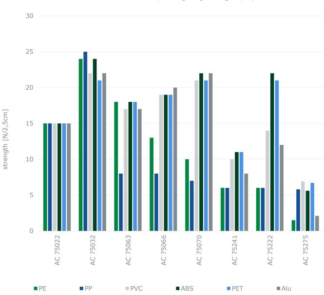
FINAT Test Method FTM 1, Coating Weight: 30 g/m<sup>2</sup>, dry
